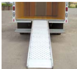
Aluminum sliding walk ramp
